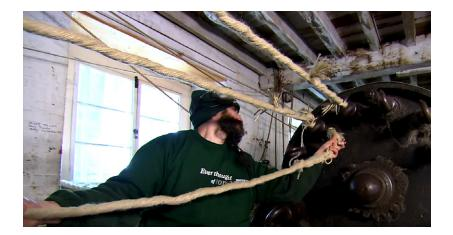
On one side, they tie three of the strands to a machine that will transform them into a rope.
