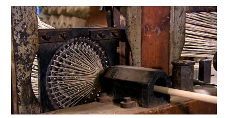
As the machine travels backward, its gears turn hooks twisting the yarns into a tight configuration.
