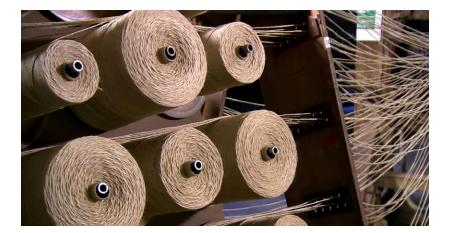
The process starts with racks of natural fiber yarns.
