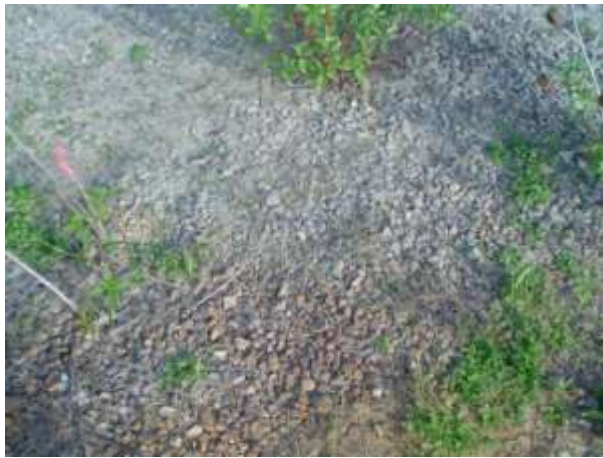
Figure 13: This figure demonstrates the affects of runoff on the gravel in Raingarden #2.
