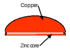
Figure 1. Cross-section of a modern (post 1983) penny.
