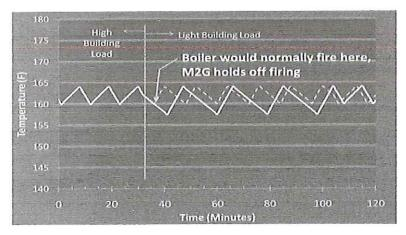
Designed by boiler experts in Europe, the M2G product is a boiler control microprocessor that determines if a real request for heat on the boiler exists, or if the boiler is dry-cycling. If it is determined that a real call exists, the boiler is immediately released to fire. If it is determined that
