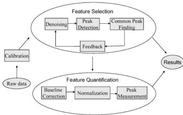
**Fig. 1.** Wave-spec package process chart.
