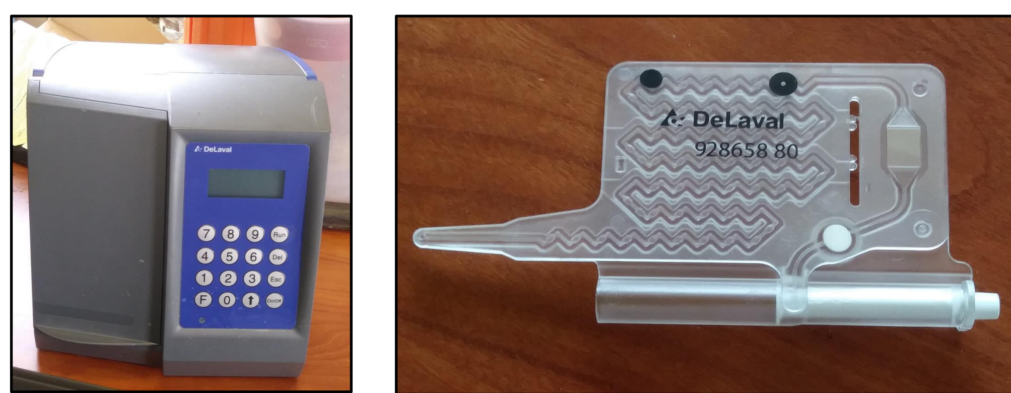
Figure 1. DeLaval Cell Counter (left) and cartridge used for SCC sample testing (right).
